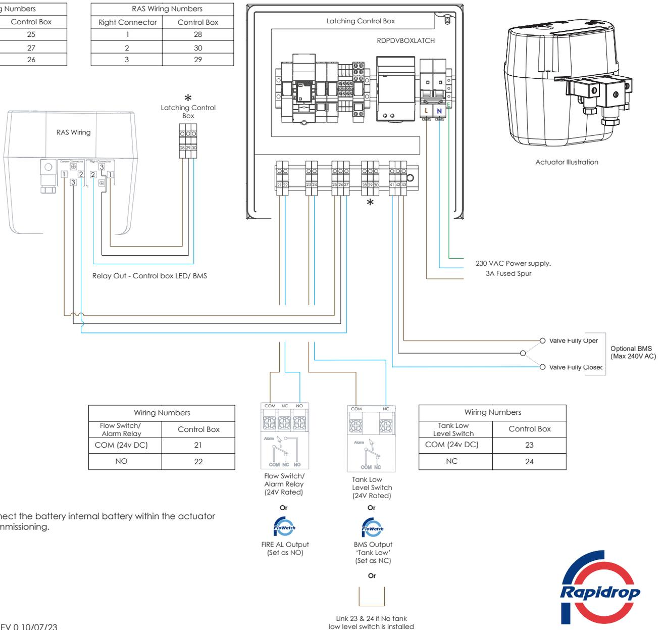
Note: Connect the battery internal battery within the actuator prior to commissioning.
