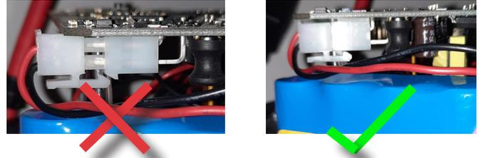
Make sure battery connection is completely in place!
