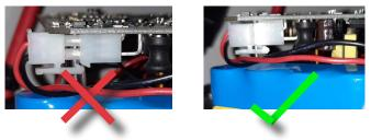
Make sure battery connection is completely in place!
