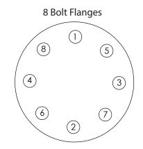
The above sequence is intended as a guide for best practise to minimise potential damage to the actuator.
