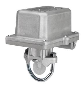
**Robust Construction:** The RDWFDEXP series consists of a rugged, NEMA 4-rated cast aluminum housing. Designed for both indoor and outdoor use, the RDWFDEXP series operates across a wide temperature range, from 32°F to 160°F. Inside, two sets of SPDT (Form C) synchronized switches are enclosed in a rugged terminal block to assure reliable performance.
