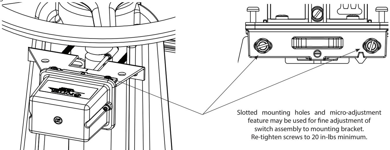
Slotted mounting holes and micro-adjustment feature may be used for fine adjustment of switch assembly to mounting bracket. Re-tighten screws to 20 in-lbs minimum.
