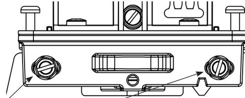
Slotted mounting holes and micro-adjustment feature may be used for fine adjustment of switch assembly to mounting bracket
