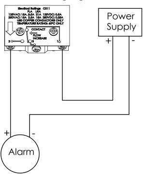
For installation instructions of the flow switch refer to Rapidrop datasheet (DS 2.13)
