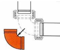
5. Coupling are non-directive and pipe can be rotated 360° during installation.
