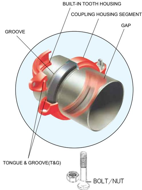
3. The T&G mechanism features a slight offset at the foot of the coupling halves which serve to protect the gasket from exposure.
