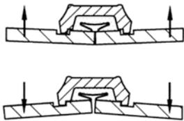
2. The C-shaped rubber gasket : provides excellent self-sealing capabilities in both low and high pressure service as well as under certain vacuum conditions.
