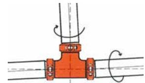
6. Coupling keys engage the full circumference of the grooves and provide significant pressure and end load restraint against pipe movement from internal and external forces.
