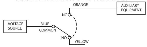
Green wire is provided as ground for the switch housing. Switch rating: 10.1Amps-125/250VAC-60Hz Actual switch application rating: 10Amps/115VAC-60Hz, 0.5Amps/28VDC
