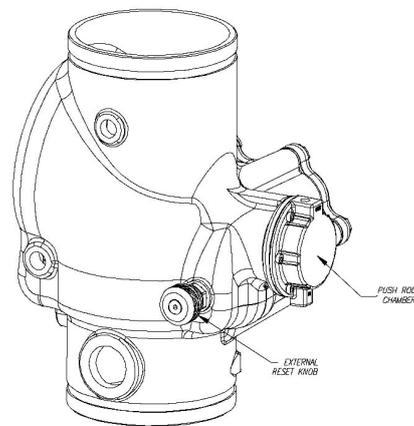
*PUSH INWARD AND ROTATE KNOB CLOCKWISE TO RESET CLAPPER. DO SO ONLY WHEN PUSH ROD CHAMBER IS VENTED.*
