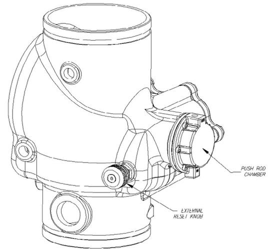
PUSH INWARD AND ROTATE KNOB CLOCKWISE TO RESET CLAPPER.
