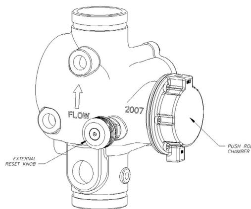
PUSH INWARD AND ROTATE KNOB CLOCKWISE TO RESET CLAPPER. DO SO ONLY WHEN PUSH ROD CHAMBER IS UNPRESSURIZED (0 PSIG).
