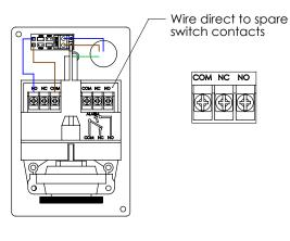
Flowswitch enables connection to alarm panel & pump controller. Refer to pump controller manufacture for NO or NC contact
